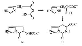
tween anhydride and isocyanate is shifted to the left when X = S. It was also possible to prepare histidyl peptides using compound 11 (X = S). The reaction proceeded slowly at room temperature but 11, unlike the NTA, failed to give histidyl peptides at an appreciable rate at 0°.
